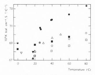
Fig. 3 — Thermal conductivity of glycerin
